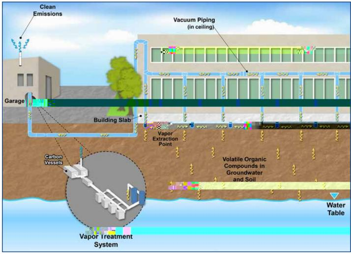
Graphic depicts sub-slab vacuum system which extracts vapors from beneath the entire building and pipes those vapors to the garage, where they are treated and clean air is released.
